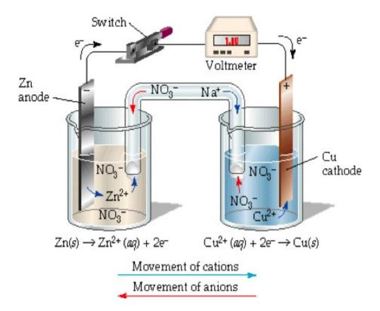
a) The oxidation half-reaction for this electrochemical cell is  $Zn \rightarrow Zn^2 + 2e^-$
